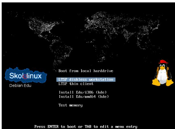
This setup also allows to boot diskless workstations and thin clients on the main network. Diskless workstations must be added with LWAT just like normal workstations or thin client servers.
